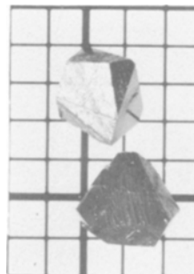
Figure 3 Octahedra of Mn_xCr_yO_4 (1 mm grid).
